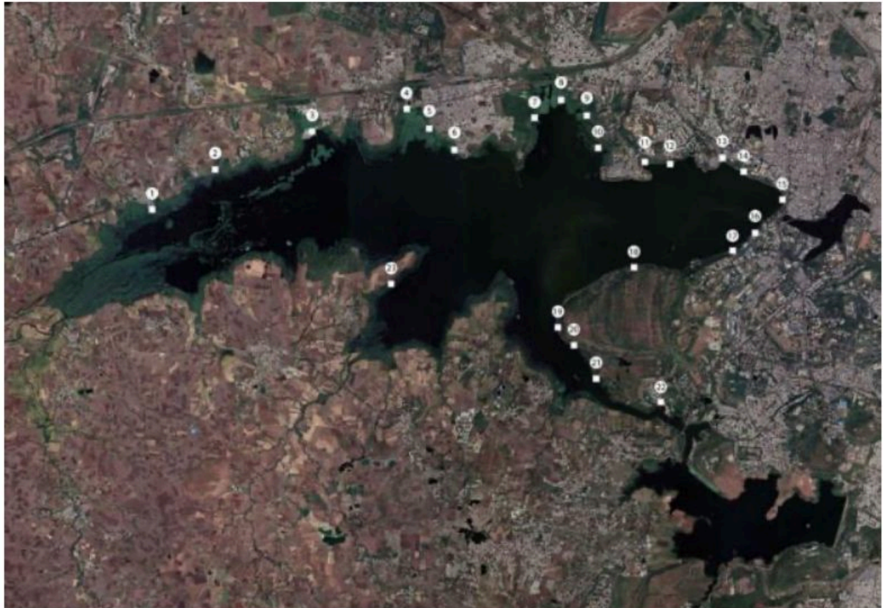
Figure 18: 22 Sewage discharge points are located through on-site interviews and observations, with some of the identifications being hypothesis-based. National Green Tribunal, however, identified a significantly higher number of operational Nallas tha
